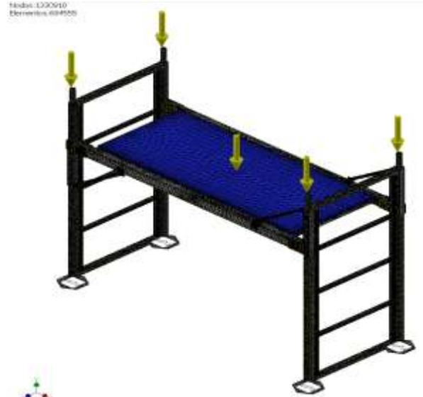
Fig. 13 Representation of the structural mesh and application of loads in the defined scenarios
