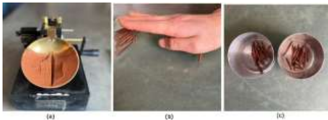
Fig. 1 Atterberg limits test on a clayey soil, (a) Determination of the liquid limit using the Casagrande cup device, (b) Rolling soil threads for the plastic limit test, and (c) Molded threads ready for oven-drying to determine their moisture content.
