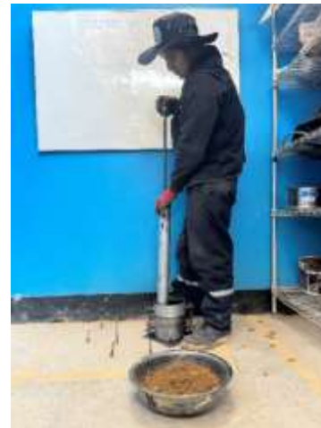
Fig. 3 Manual execution of the modified proctor with a standard tamper on the sample in molds
