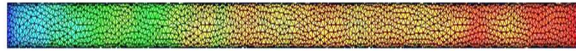
Fig. 5 CFD mesh of the oval tube model, with localized refinement in curvature zones to capture thermal gradients more accurately
