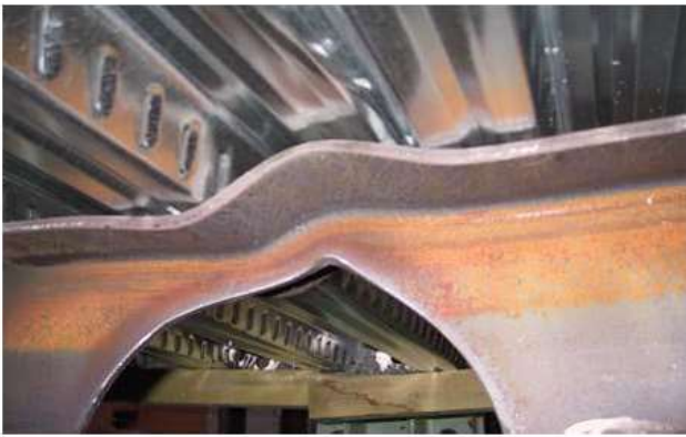
Fig. 8 The Mechanism of Vierendeel [48]
