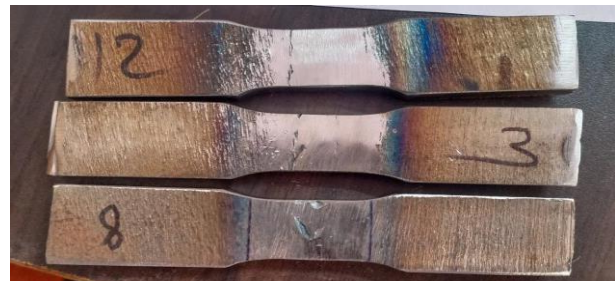
Fig. 3 (a) Specimen before tensile test
